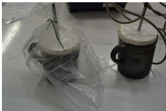
Figure 3. Experiment which can show the heat loss by water evaporation inside the unglazed clay mug
