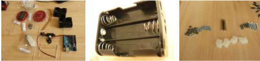
Figure 10. Arduino kit for the construction of a robot
