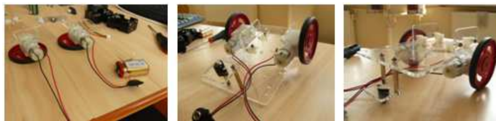
Figure 12. Securing the assembly wheels-motors on the chassis
