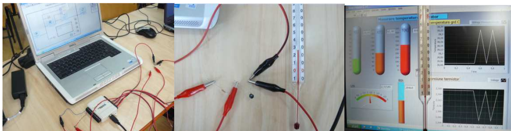
Figure 4. Laboratory temperature monitoring, R_{th}=28,5\text{kohms} , t=28,04^{\circ}\text{C}
